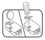
4. Replace the battery cover and tighten the screw to secure.
